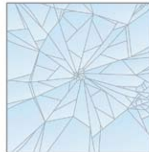
Example of fragmentation of laminated glass
